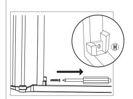
Using a Philips screwdriver, remove the screw holding the One-Way Stopper (H) in place.
