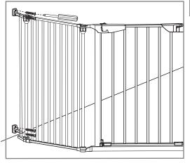
10. Tighten each Tension Knob (D) to secure the position.
